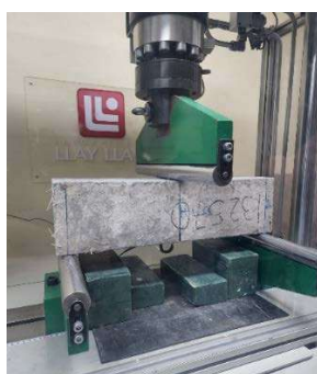
Figure 1: The beam test setup was performed according to EN 14651
