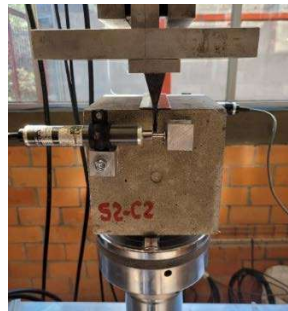
Figure 2: Cube test setup according to the Montevideo method
